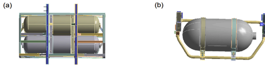
Fig. 3. Fixed constraint application surface of the onboard hydrogen storage system: (a) Commercial vehicle onboard hydrogen storage system, (b) Passenger vehicle onboard hydrogen storage system.
